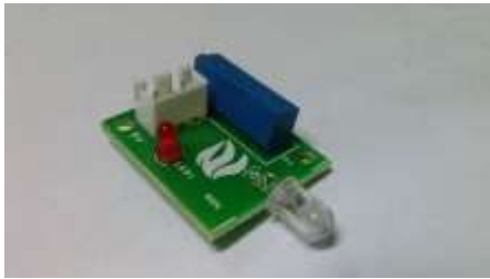
FIG . Fire sensor
